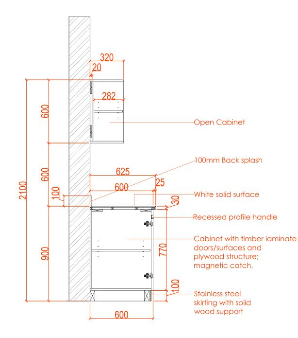
PRINTER UNIT. SECTIONAL Details-A PRINTER UNIT. SECTIONAL Details-B
